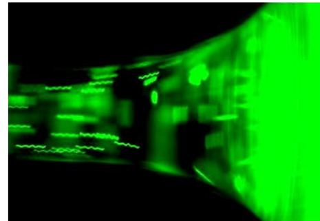
Mechanochemistry: Extensional strain drives collagen fibrillogenesis. Fluorescence images show strain field in fluid ACSNano 2016
